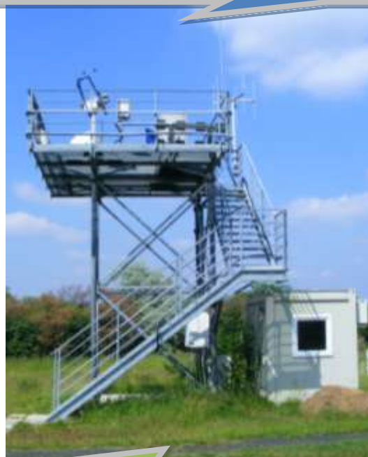
Solar radiation measure platform
